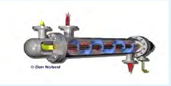
Heat exchangers leaks (externally and between the streams) can be detected through temperature/pressure relation changes and Heat/mass balances [Swan, 2006]
