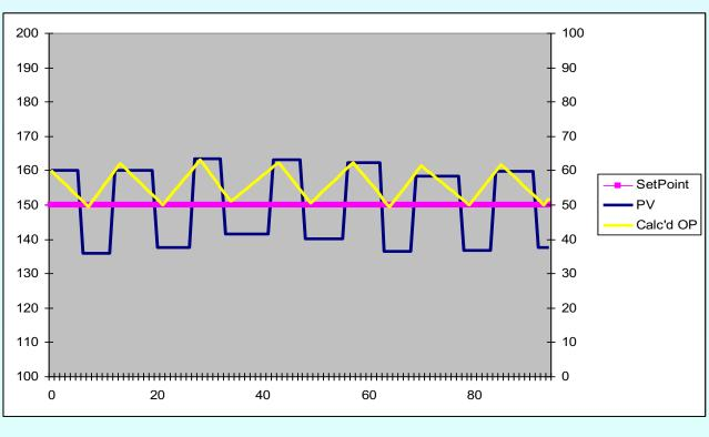
Controller output (CO) and process variable (PV) curves are out of phase and display a saw tooth pattern for sticky control valves [Swan, 2006]
